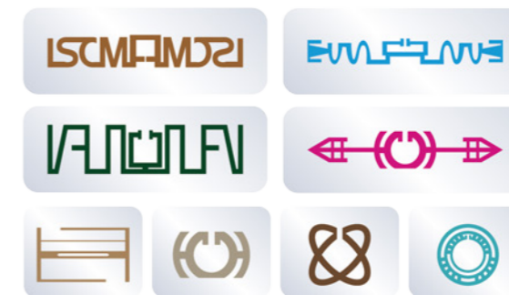
Tag antenna optimised for lossy dielectrics with medium permittivity (e.g. soil, wine bottle)
